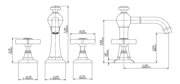
The measurements shown are for reference only. Products and specifications shown are subject to change without notice. Revised 5/2018. <u>www.graff-designs.com</u> | phone: 800-954-4723 BATHROOM Camden Deck-Mounted Handshower & Diverter Set G-6955-C16B
