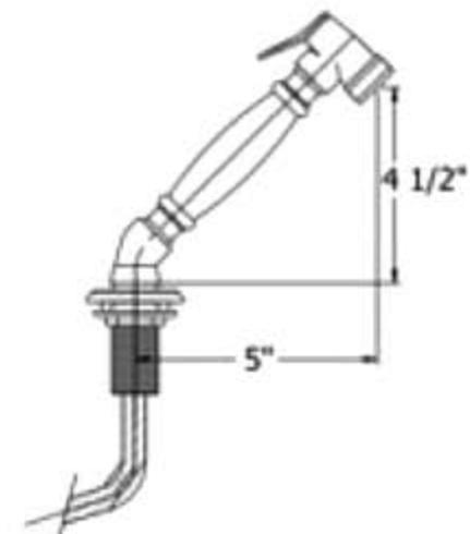
Body Installation Hole  $\text{O } 1 \frac{3}{4}"$  Spray Installation Hole  $\text{O } 1 \frac{3}{8}"$
