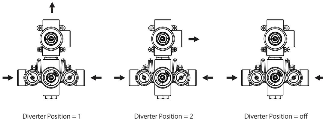
**TVH.4420 | 3/4" Thermostatic Valve With 2-Way Diverter & Integrated Volume Control** Page 1 of 2
