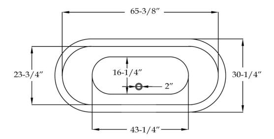
Weight (empty): 445 lbs Weight (filled): 9070 lbs Capacity: 55 gal Water depth: 15"
