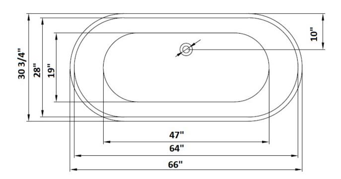
The Overflow channel is molded into the interior tub wall. Drain is included. Please use a bead of silicone around the base of the tub to provide a seal between the tub and the floor, and to prevent the tub from moving.
