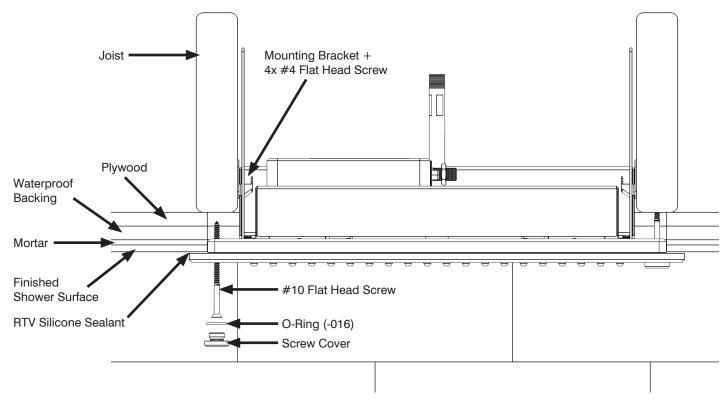
(Fig. 1) Installation Profile View
